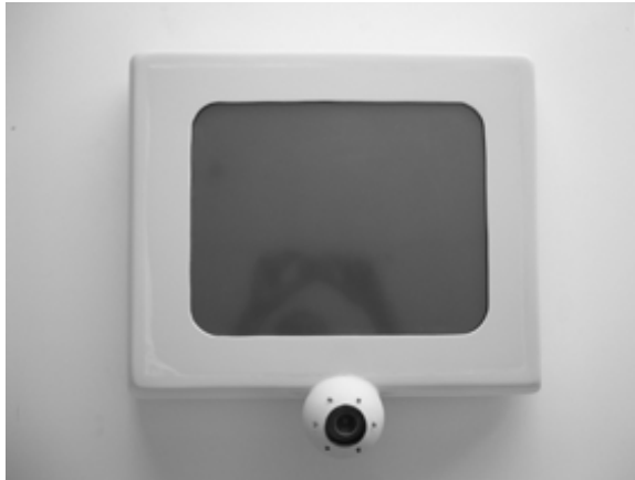
Fig. 3. A "transparent" representation for an ubiquitous computing component: a touchscreen enhanced with perceptive capability due to the embedded webcam
